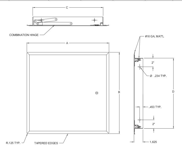
STANDARD FEATURES: SLOTTED SCREWD CAM LATCH, CARBON STEEL, BAKED WHITE PRIME COAT (ADDITIONAL FINISH PAINT IS RECOMMENDED FOR SUPERIOR CORROSION RESISTANCE).
