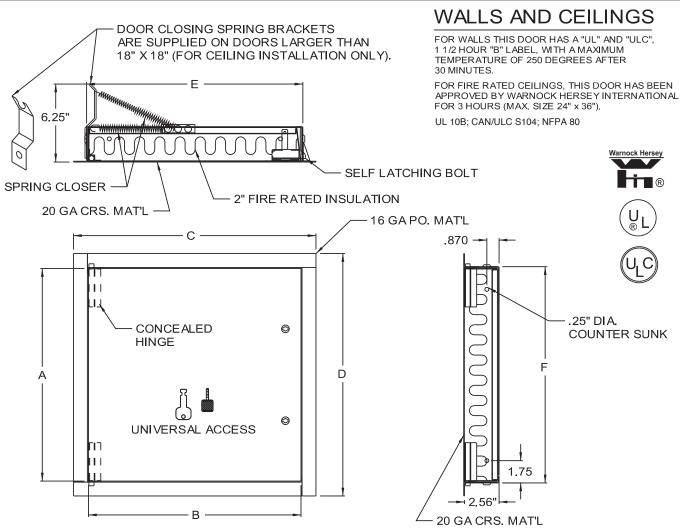
STAND ARD FEATURES: UNIVERSAL SELF LATCHING BOLT- OPERATED BY KNURLED KNOB/ FLUSH KEY, WITH INSIDE TURN RELEASE. CARBON STEEL BAKED WHITE PRIME COAT (ADDITIONAL FINISH PAINT IS RECOMMENDED FOR SUPERIOR CORROSION RESISTANCE). **OPTIONS:**
