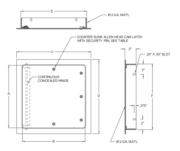
STAND ARD FEATURES: TAMPER RESISTANT ALLEN HEAD CAM LATCH WITH SECURITY PIN, CARBON STEEL, BAKED WHITE PRIME COAT (ADDITIONAL FINISH PAINT IS RECOMMENDED FOR SUPERIOR CORROSION RESISTANCE).
