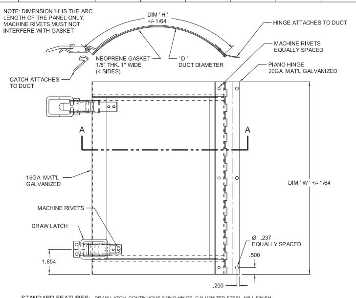
STANDARD FEATURES: DRAW LATCH, CONTINUOUS PAINO HINGE, GALVANIZED STEEL, MILL FINISH
